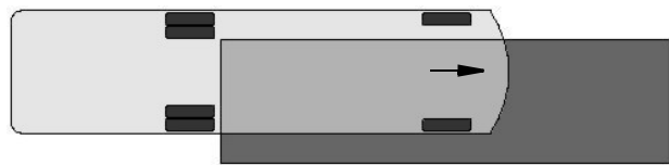
Weighing Right Front Corner
