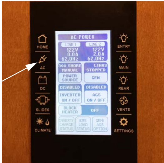
Generator Switch and Hourmeter (Located on multiplex monitor panel "AC" Screen) -Typical View
