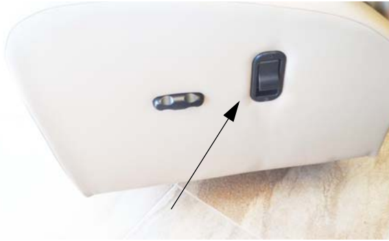
Co-Pilot Footrest Lever (Located on inboard side of co-pilot seat) -Typical View
