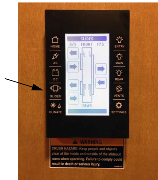
Slideout Switch (Located on Multiplex Monitor Panel) -Typical View
