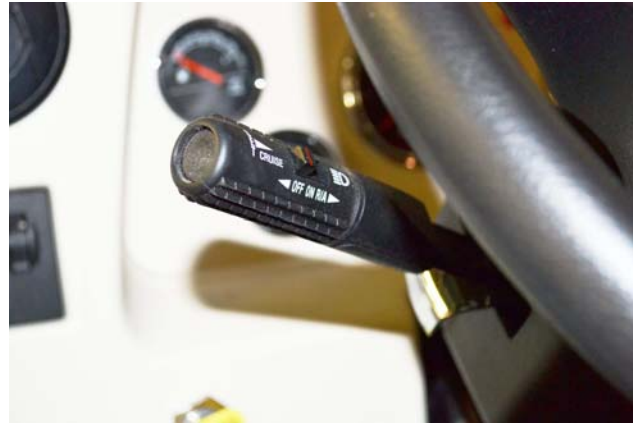
Turn Signals/High-Low Beams (Typical View - your motorhome may differ depending on model)
