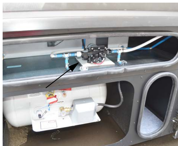
Water Pump (Located in driver side front compartment) *Model 34T
